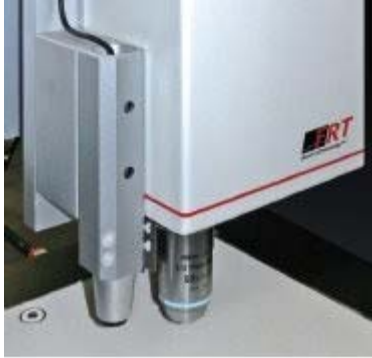
Figure 5 - FRT's open architecture combines field-of-view confocal microscopy (right objective) with a chromatic white light confocal point sensor (left) for large area raster scans.
